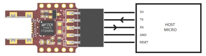
The micro USB is designed to have a compact footprint, and be compatible with prototyping such as plugging it directly into a breadboard when male 2.54mm (0.1") headers are soldered to the row of 5 pins, along each side.
