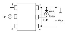
Fig. 13.1.1 I<sub>OPH</sub> Test Circuit
