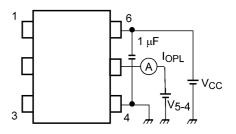
Fig. 13.1.2 I<sub>OPL</sub> Test Circuit
