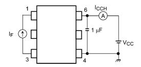
Fig. 13.1.5 I<sub>CCH</sub> Test Circuit
