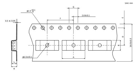
Table Tape Dimensions (unit: mm, tolerance: ±0.1)
