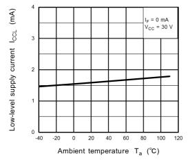
Fig. 13.2.5 I<sub>CCL</sub> - T<sub>a</sub>
