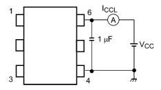
Fig. 13.1.6 I<sub>CCL</sub> Test Circuit
