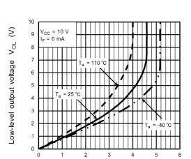
Peak low-level output current  $I_{OPL}$  (A) Fig. 13.2.9  $V_{OL}$  -  $I_{OPL}$
