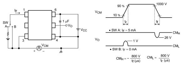
Fig. 13.1.8 Common-Mode Transient Immunity Test Circuit and Waveform
