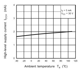
Fig. 13.2.6 I<sub>CCH</sub> - T<sub>a</sub>
