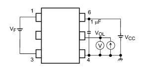
Fig. 13.1.4 V<sub>OL</sub> Test Circuit
