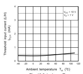
Fig. 13.2.4 I<sub>FLH</sub> - T<sub>a</sub>
