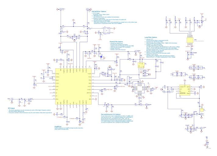
Figure 5-1. LMX2541 EVM Schematic
