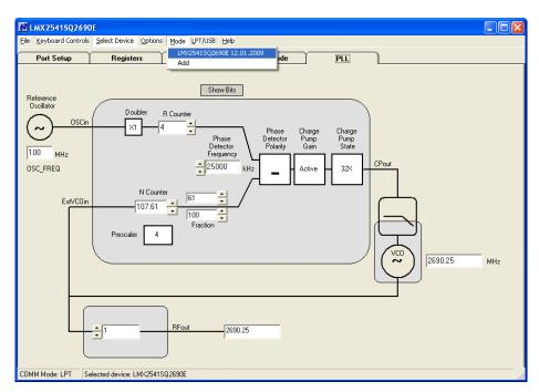
Figure 2-9. LMX2541SQ2690E Code Loader Settings
