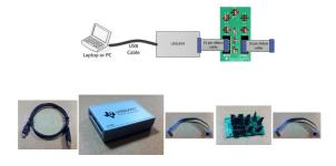
Figure 7-2. USB2ANY-uWire Adapter Board
