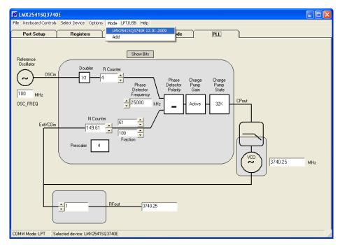
Figure 2-15. LMX2541SQ3740E Code Loader Settings
