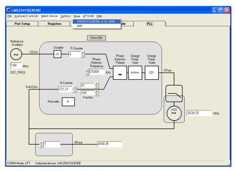
Figure 2-11. LMX2541SQ3030E Code Loader Settings
