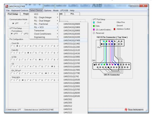
Figure 2-2. Selecting Device in Code Loader
