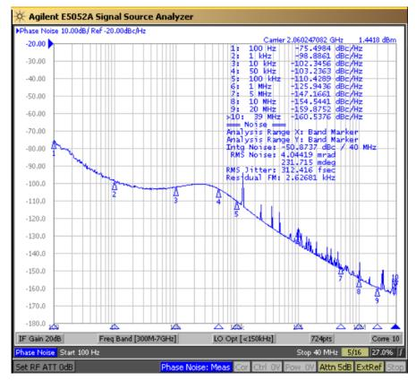
Figure 2-6. LMX2541SQ2060E Measured Performance
