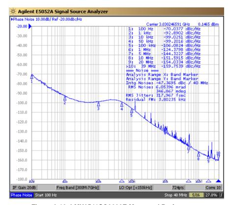
Figure 2-12. LMX2541SQ3030E Measured Performance
