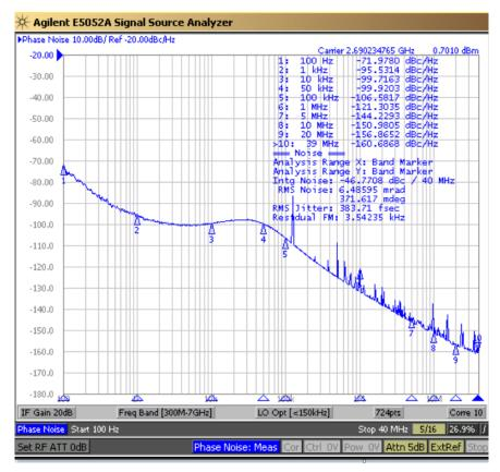
Figure 2-10. LMX2541SQ2690E Measured Performance
