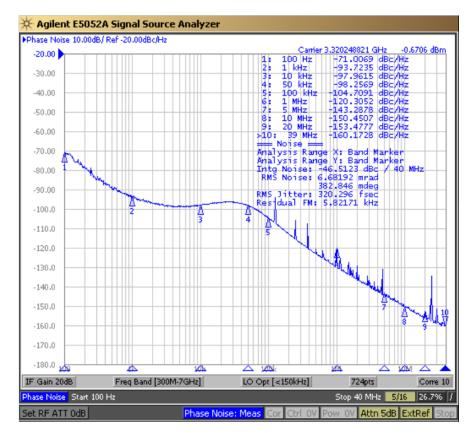
Figure 2-14. LMX2541SQ3320E Measured Performance
