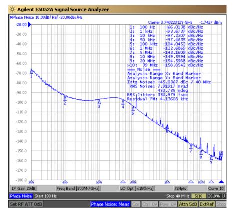
Figure 2-16. LMX2541SQ3740E Measured Performance
