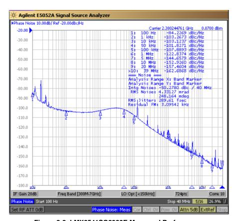
Figure 2-8. LMX2541SQ2380E Measured Performance
