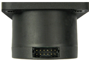
Fig. 1 Hirose DF11-12DP-2DS9(24) header
