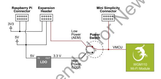
Figure 4.5. WGM110 Wi-Fi Expansion Kit Power Topology
