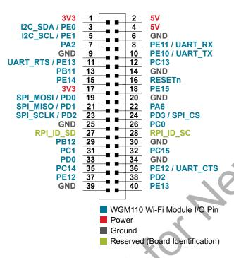
Figure 4.3. Raspberry Pi Connector
