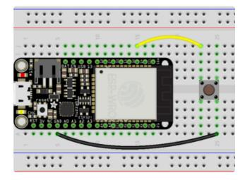
Feather GND to Push Button Feather GPIO D14 to Push Button Note - we are not using a resistor part! We will be configuring the Feather ESP32 to use its internal resistor instead.
