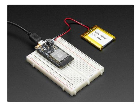
Comes fully assembled and tested, with a USB interface that lets you quickly use it with the Arduino IDE or the low-level ESP32 IDF. We also toss in some header so you can solder it in and plug into a solderless breadboard.
