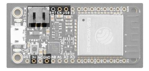
• GND - this is the common ground for all power and logic
