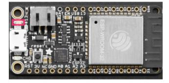
The Adafruit HUZZAH 32's LED (highlighted in red) is located next to the micro-USB connector.
