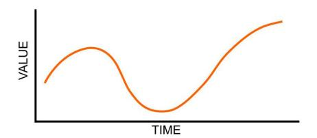
Analog signals are continuous values which means they can be an infinite number of different voltages. Think of analog signals like a floating point or fractional number, they can smoothly transiting to any in-between value like 1.8V, 1.81V, 1.801V, 1.8001V, 1.80001V and so forth to infinity.
