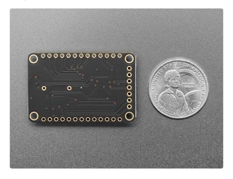
The IS31FL3731 is a nice little chip - it can use 2.7-5.5V power and logic so it's flexible for use with any microcontroller. You can set the address so up to 4 matrices can share an I2C bus. Inside is enough RAM for 8 separate frames of display memory, so
