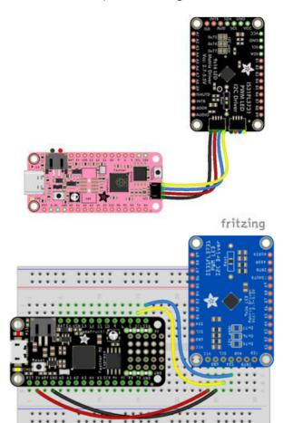
Board 3V to breakout VCC Board GND to breakout GND Board SCL to breakout SCL Board SDA to breakout SDA
