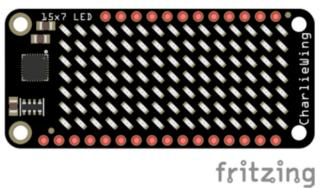
Assemble the CharlieWing by soldering headers onto the board.
