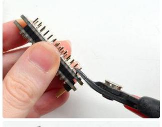
Now you can trim the long header with diagonal cutters. Cut one or two pins at a time
