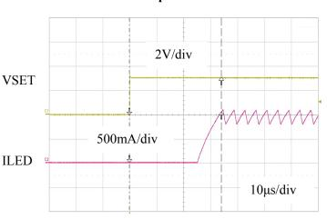
Dimming Waveforms (PWM=50%, 3LEDs, 100 $\mu$ H, Vin=16V,Rs=0.33 $\Omega$ )
