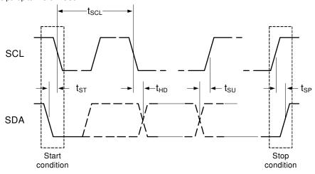
Figure 2: I<sup>2</sup>C Data Transfer
