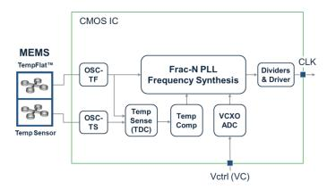
Figure 47. Block Diagram - VCTCXO
