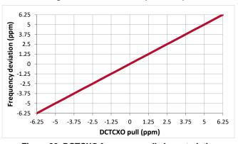
Figure 38. DCTCXO frequency pull characteristic
