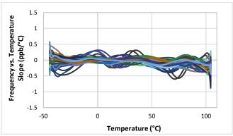
Figure 24. Freq. vs. Temp. Slope (ΔF/ΔT)
