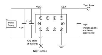
Figure 10. LVCMOS Test Circuit (NC Function)
