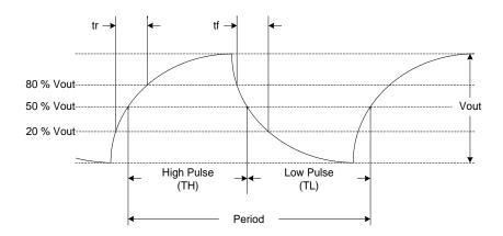
Figure 16. Clipped Sinewave Waveform Diagram<sup>[14]</sup>
