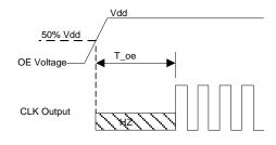
T\_oe: Time to re-enable the clock output
