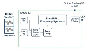
Figure 46. Block Diagram - TCXO
