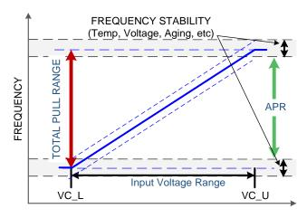
Figure 51. Typical SiTime VCTCXO FV Characteristic
