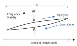
Figure 19. Illustration of hysteresis, where  $\Delta F$  is max frequency difference between up and down cycles across temperature
