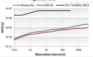
Figure 22. MTIE (0.1 Hz loop bandwidth) [15]
