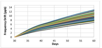
Figure 27. Frequency drift after 30 days [16]
