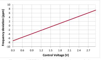
Figure 23. VCTCXO frequency pull characteristic
