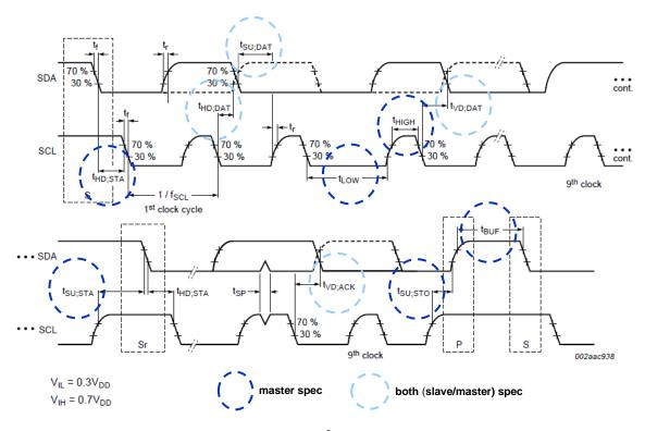
Figure 59. I<sup>2</sup>C Timing Diagram
