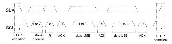
Figure 57. Parallel data byte format, read operation
