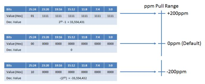
Figure 52. Pull Range and Frequency Control Word
