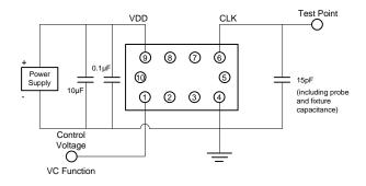
Figure 8. LVCMOS Test Circuit (VC Function)
