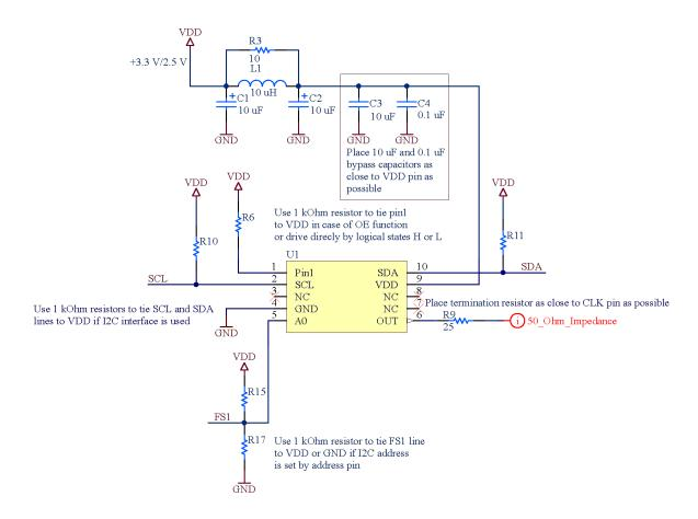
Figure 60. DCTCXO schematic example
