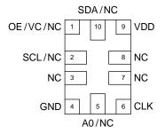
Figure 2. Pin Assignments (Top view)
