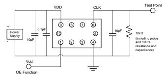
Figure 6. LVCMOS Test Circuit (OE Function)
