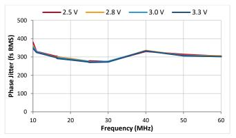
Figure 37. RMS Phase Jitter, VCTCXO (LVCMOS)
