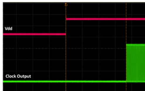
Figure 16. Startup Waveform vs. Vdd
