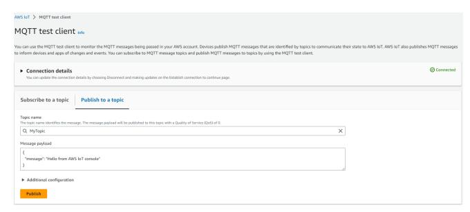
Figure 4: Publish to a Topic on MQTT test client in AWS IoT console
