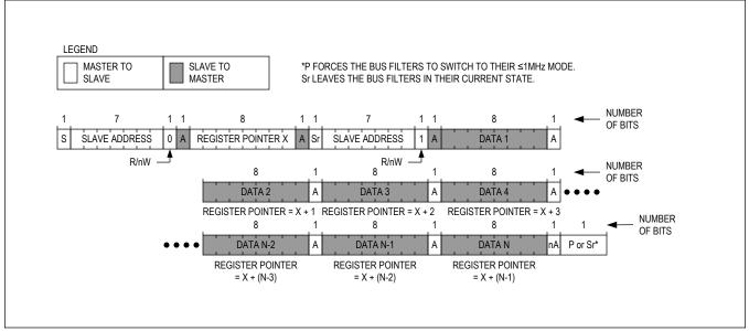
Figure 13. Reading from Sequential Registers
