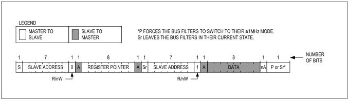
Figure 12. Reading from a Single Register
