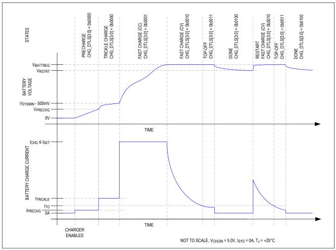
Figure 1. Li Battery Charge Profile
