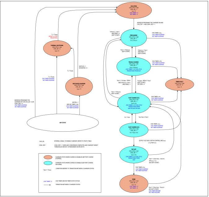
Figure 2. Charger State Diagram
