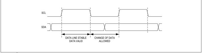
Figure 7. I<sup>2</sup>C Bit Transfer
