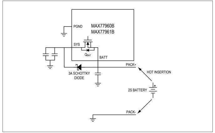
Figure 14. Battery Insertion Protection with 2S Battery
