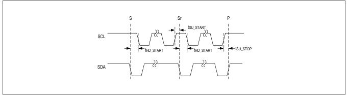
Figure 8. I<sup>2</sup>C Start Stop
