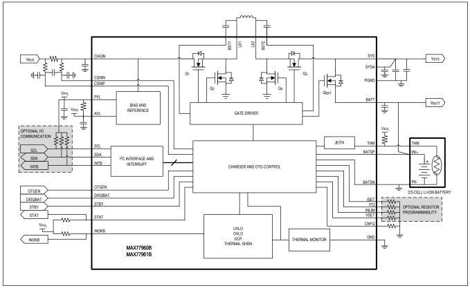
25V<sub>IN</sub>, 3A<sub>OUT</sub> to 6A<sub>OUT</sub>, USB-C Buck-Boost Charger with Integrated FETs for 2S/3S Li-Ion Batteries
