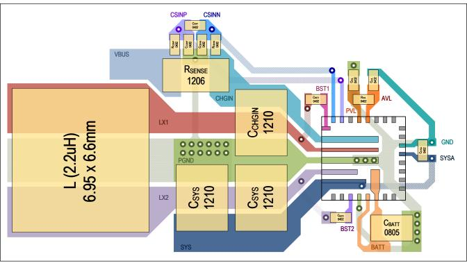
Figure 16. PCB Layout Example
