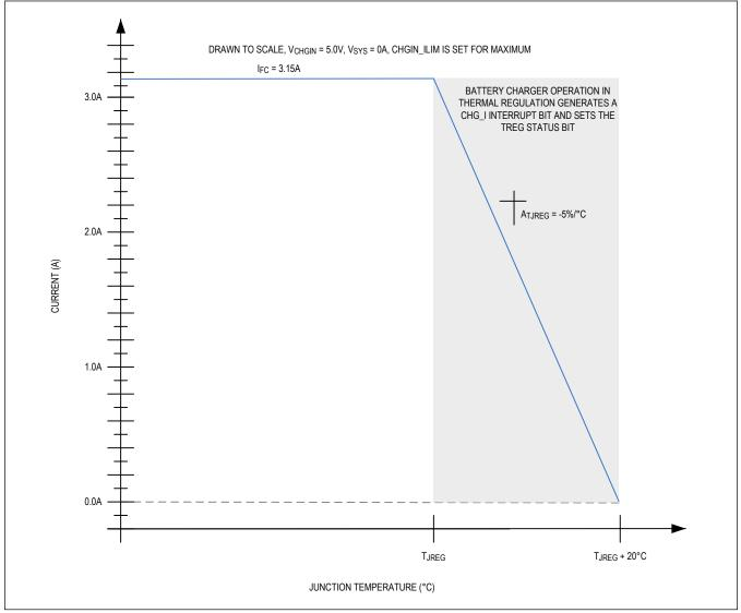
Figure 3. Charge Currents vs. Junction Temperature
