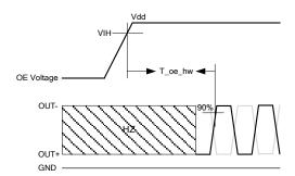
Figure 8. Hardware OE Enable Timing
