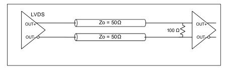
Figure 14. LVDS Single DC Termination at the Load
