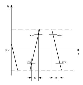
Figure 7. LVDS Differential Waveform (i.e. OUT+ minus OUT-)
