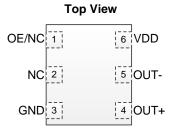
Figure 3. Pin Assignments
