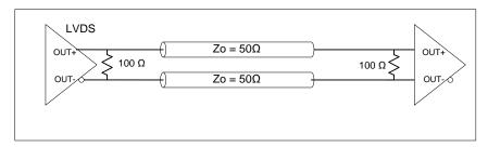
Figure 16. LVDS Double DC Termination
