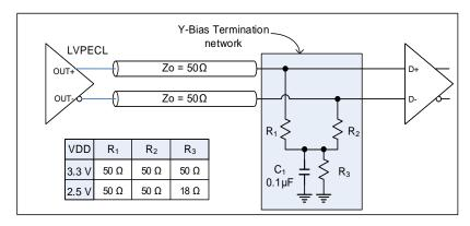
Figure 12. LVPECL and Low-swing LVPECL with Y-Bias Termination
