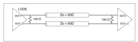
Figure 16. LVDS Double DC Termination
