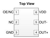
Figure 3. Pin Assignments
