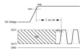
Figure 8. Hardware OE Enable Timing
