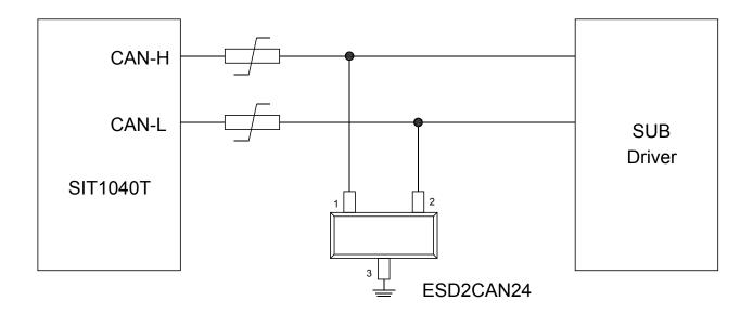
Typical Interface Application of CAN Bus Protection
