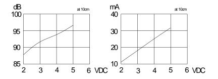
Temperature :  $20 \pm 3$  °C Relative humidity : 60%  $^{\sim}$  70%, Atmospheric pressure : 860mbar to
