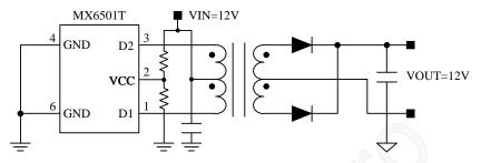
Application 2: 12V input converter to 12V with a resistor divider for VCC supply
