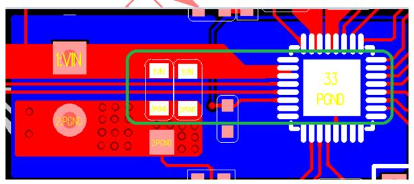
3. As shown in the following figure: Sampling routes from current sampling resistors to IP6806 ISENSE and IGND need separate leads from both ends of resistors, not to coincide with the power routes of the same network
