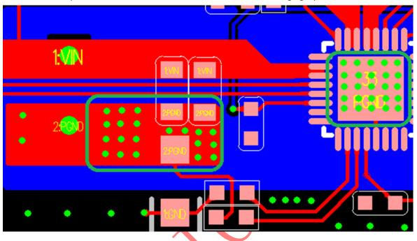
2. As shown in the following figure: input the filter capacitance between VIN and PGND, the smaller the ring road area, the better;
