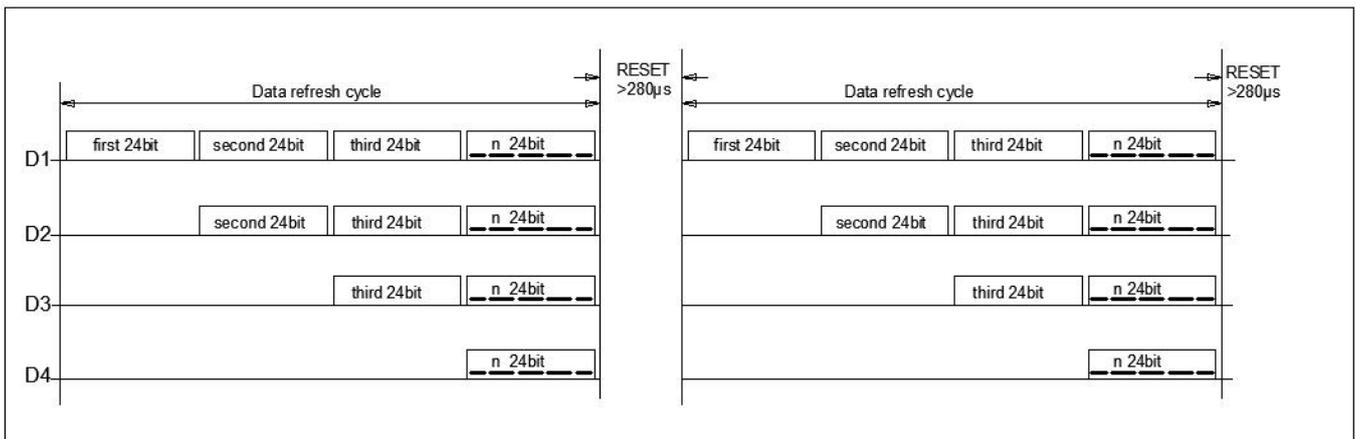
Note: The data of D1 is send by MCU, and D2, D3, D4 through IC internal reshaping amplification to transmit.
