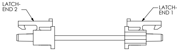
-LUS [LATCH UP- CABLE STRAIGHT]
