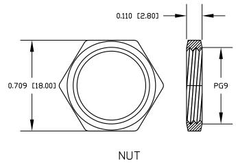
NOTE: MATERIAL HDUSING: PBT UL94V-0, BLACK CONTACT: **BRASS** NUT: **BRASS** SHELL: **BRASS** D-RING: EPDM, BLACK **FINISH** CONTACT: GOLD PLATED, 10 µ" Min. UNDER PLATE: NICKEL NICKEL PLATED NUT: SHELL: NICKEL PLATED **ELECTRICAL** RATED CURRENT: 4A RATED VOLTAGE: 250V INSULATION RESISTANCE: 100ΜΩ ΜΙΝ CONTACT RESISTANCE:  $10m\Omega$  MAX WATER PROOF: IP67/68 **ENVIRONMENT**
