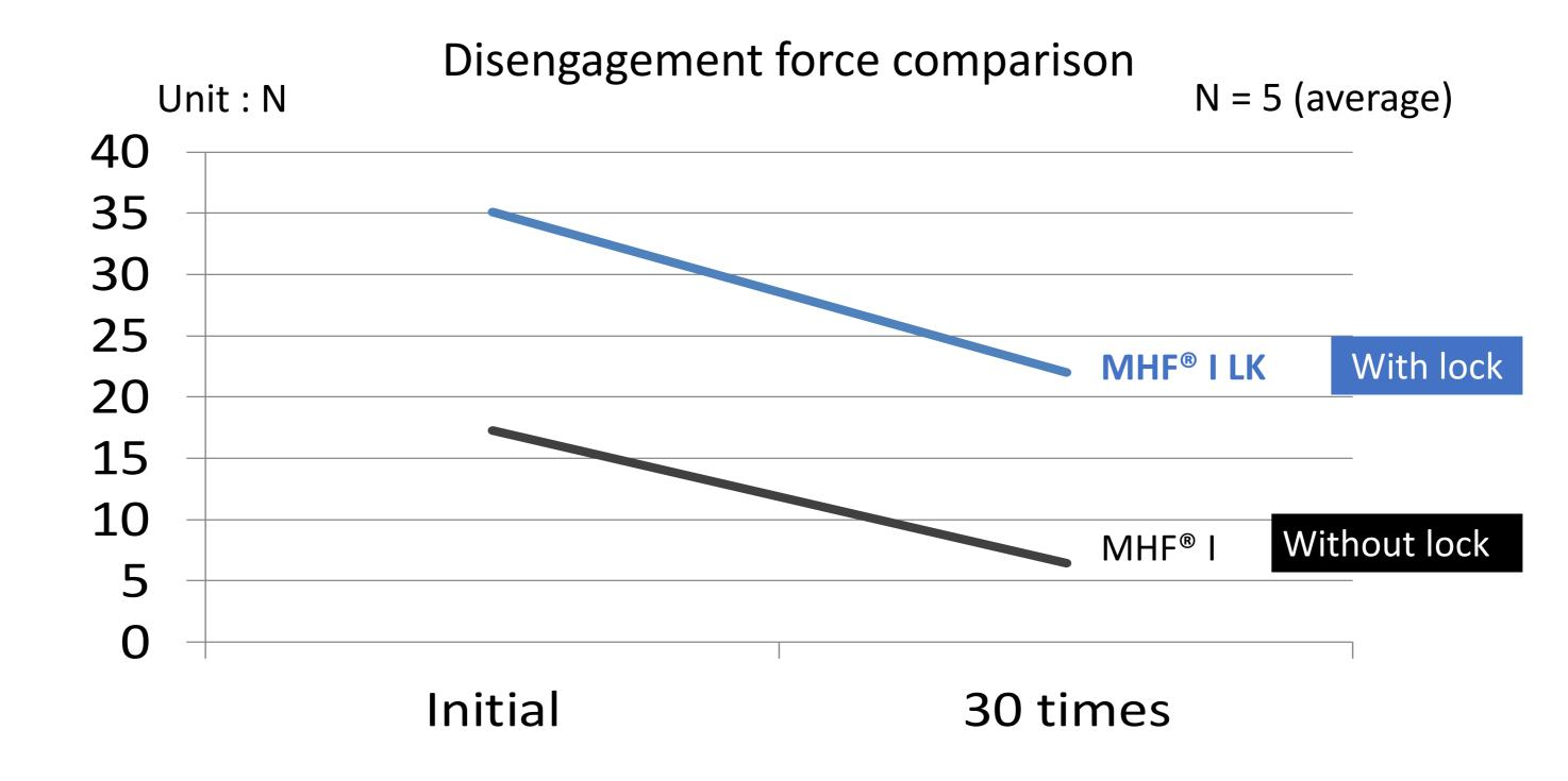
Patented locking system for MHF<sup>®</sup> I plug
