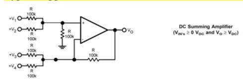
Where:  $V_0 = V_1 + V_2 - V_3 - V_4$ ,  $(V_1 + V_2) \ge (V_3 + V_4)$  to keep  $V_0 \ge 0$   $V_{DC}$
