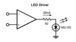
$V_0 = 0 \ V_{DC}$  for  $V_{IN} = 0 \ V_{DC}$ ,  $A_V = 10$
