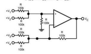
Where:  $V_0 = V_1 + V_2 - V_3 + V_4$ ,  $(V_1 + V_2) \ge (V_3 + V_4)$  to keep  $V_0 \ge 0$   $V_{DC}$
