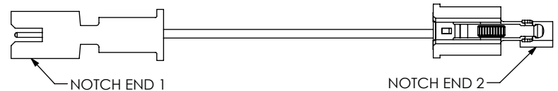
TR-NDS (END 2 NOTCH DOWN, CABLE STRAIGHT) (PIN 1 TO PIN 1)
