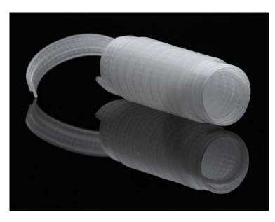
Gamma's Clear SDL Cold Shrink Tubingis a specially formulated, pre-expanded transparent silicone rubber shrink tubing that does not require heat to shrink. It is intended for weatherproofing of AC & DC electrical power wire/lug assemblies. This transparent silicone rubber allows the integrity of the waterproof seal on the wire/lug interface to be
