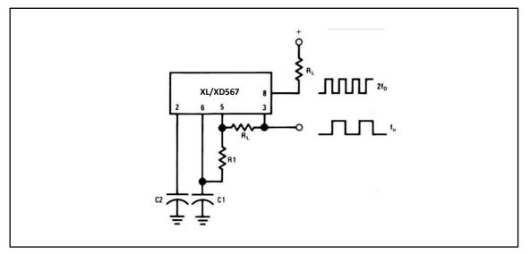
Figure 8-5. Oscillator with Double Frequency Output
