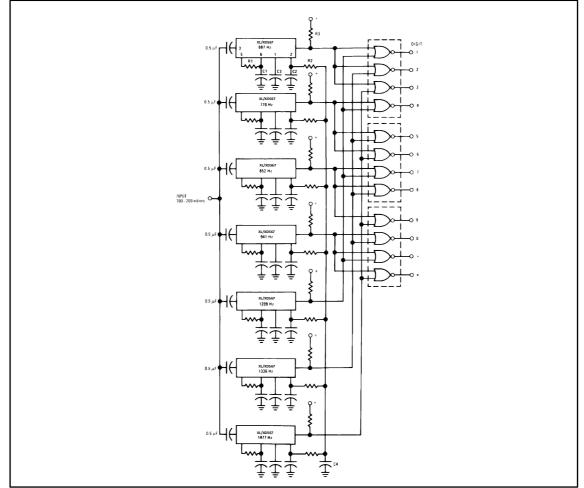
Component values (typ) R1 6.8 to 15k R2 4.7k R3 20k C1 0.10 mfd C2 1.0 mfd 6V C3 2.2 mfd 6V C4 250 mfd 6V
