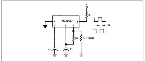
Connect Pin 3 to 2.8V to Invert Output
