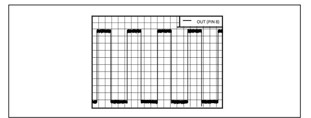
Figure 10-8. Output for 100-mA Load
