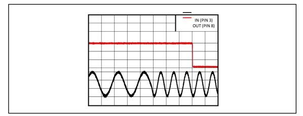
Figure 8-2. Frequency Detection
