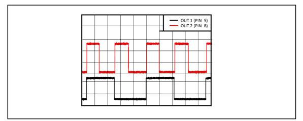
Figure 8-6. Double Frequency Output
