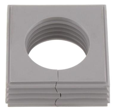
Seal, Mounting type: Plug in, Length x width: 42.8 mm, Max. cable diameter: 28 mm, IP 66, Colour: Grey
