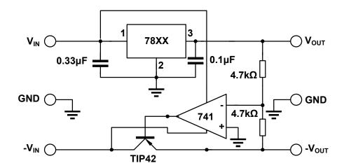
Figure 9-14. Tracking Voltage Regulator
