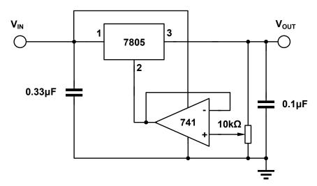
Figure 9-13. Adjustable Output
