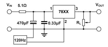
Figure 9-7. Ripple Rejection
