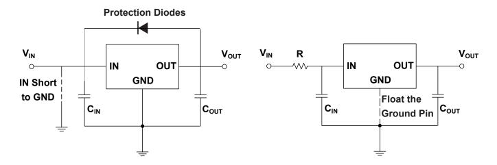
Figure 9-3. Regulator Input Short Circuit
