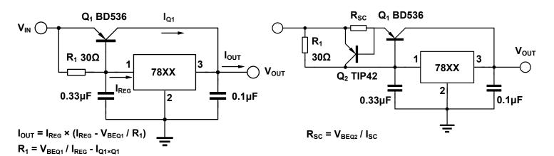
Figure 9-11. High Current with Voltage Regulator
