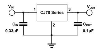
Figure 2-1. Fixed Output Voltage Regulator
