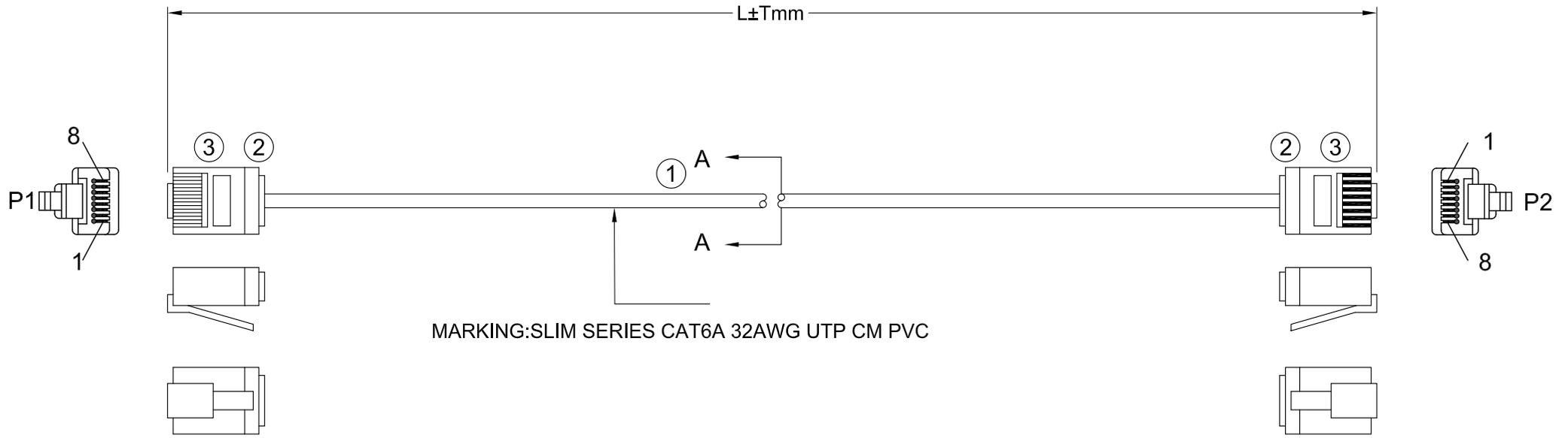
MARKING: SLIM SERIES CAT6A 32AWG UTP CM PVC
