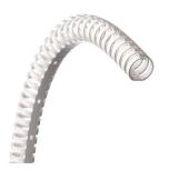
Highly flexible design saves space and allows bending at angles above 90 degrees, making it well suited for confined spaces. Overlapping circular fingers eliminate need for a separate cover to retain wires and make insertion and removal of wires fast and easy.
