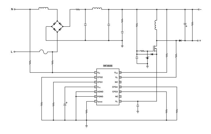
Figure 3.1 : iW3688 Simplified Application Circuit
