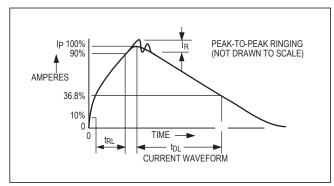
Figure 9. Human Body Current Waveform
