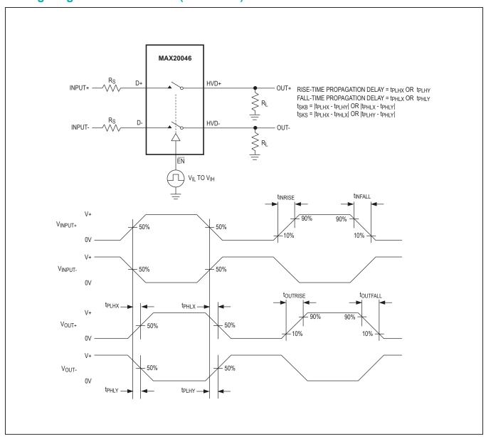
Figure 7. Propagation Delay and Output Skew
