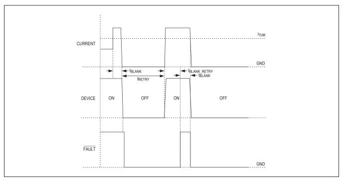
Figure 4. Timing Diagram for Overcurrent Protection
