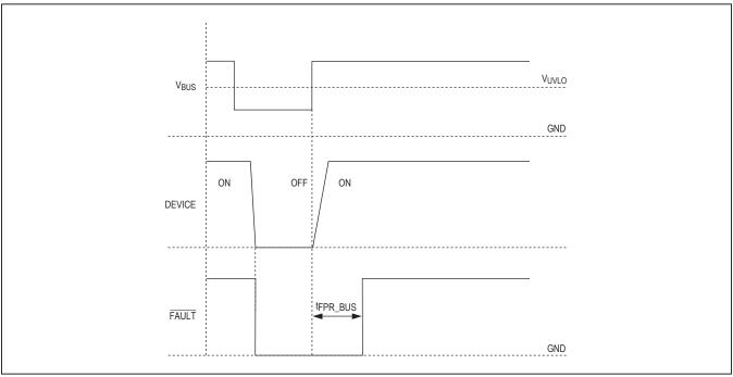
Figure 1. Timing Diagram for Undervoltage Lockout on BUS
