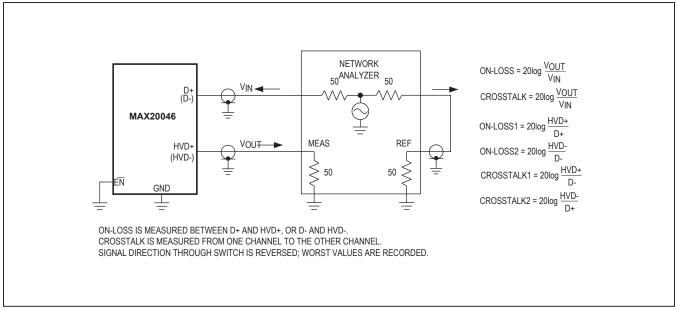
Figure 5. On-Channel -3dB Bandwidth and Crosstalk
