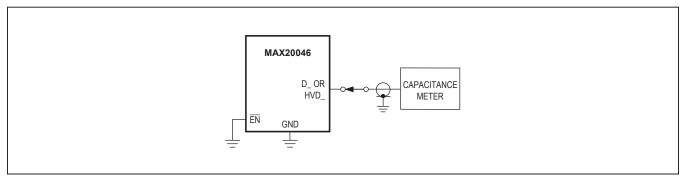
Figure 6. On-Capacitance
