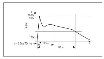
Figure 10. IEC 61000-4-2 ESD Test Model
