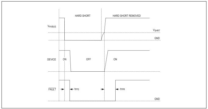
Figure 3. Timing Diagram for Short-to-Ground Protection
