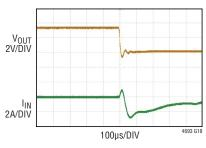
$V_{IN}$  = 3.3V,  $V_{OUT}$  = 3.3V,  $f_{SW}$  = 1MHz, 2A LOAD  $C_{OUT}$  = 3× 22 $\mu F$  + 3× 2.2 $\mu F$  CERAMIC
