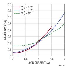
Figure 7. Power Loss at 3.3V Output and 1MHz Switching Frequency
