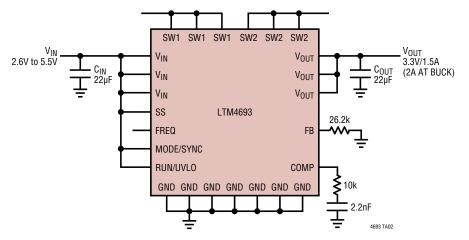
Figure 16. 2.6V to 5.5V Input, 3.3V Output with Minimum Components (Default 2ms Soft-Start Time and 1MHz Switching Frequency)
