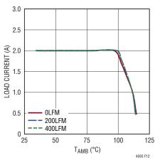
Figure 12. 5V to 1.8V Derating Curve, No Heat Sink
