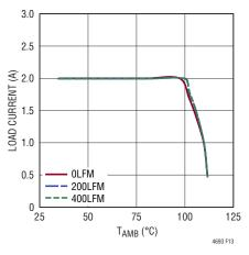
Figure 13. 5V to 3.3V Derating Curve, No Heat Sink
