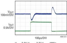
$<sup>\</sup>begin{array}{l} V_{IN}=3.3 V, \, V_{OUT}=3.3 V, \, f_{SW}=1 MHz \\ C_{OUT}=2 \times 22 \mu F \, CERAMIC \, CAP \\ C_{TH}=2200 p F, \, R_{TH}=10 k \\ LOAD \, STEP \, 1A-2A \end{array}$
