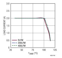
Figure 9. 3.3V to 1.8V Derating Curve, No Heat Sink
