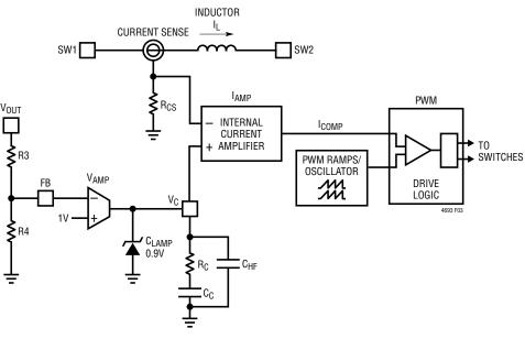
Figure 3. Average Current Mode Control Loop
