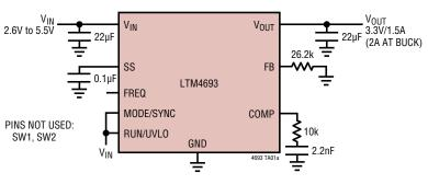
3.3V<sub>OUT</sub>, 2A DC/DC µModule Regulator
