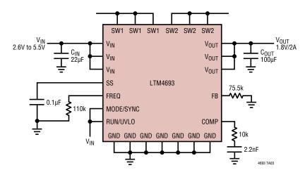
Figure 17. 2.6V to 5.5V Input, 1.8V Output with Adjustable SS Time and 2MHz Switching Frequency
