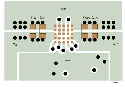
Figure 15. Recommended PCB Layout
