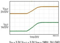
$V_{IN}$  = 3.3V,  $V_{OUT}$  = 3.3V,  $f_{SW}$  = 1MHz, 2A LOAD  $C_{OUT}$  = 3× 22 $\mu$ F + 3× 2.2 $\mu$ F CERAMIC SOFT-START CAPACITOR = 0.01 $\mu$ F USE RUN PIN TO CONTROL START-UP
