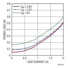
Figure 6. Power Loss at 1.8V Output and 1MHz Switching Frequency
