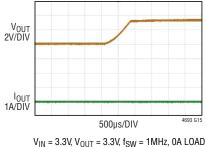
$V_{IN}$  = 3.3V,  $V_{OUT}$  = 3.3V,  $f_{SW}$  = 1MHz, 0A LOAD  $C_{OUT}$  = 3x 22µF + 3x 2.2µF CERAMIC SOFT-START CAPACITOR = 0.01µF USE RUN PIN TO CONTROL START-UP
