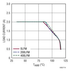
Figure 14. 5V to 5V Derating Curve, No Heat Sink
