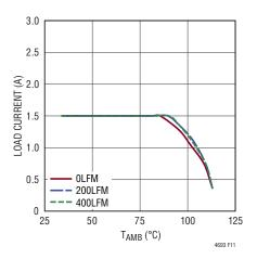
Figure 11. 3.3V to 5V Derating Curve, No Heat Sink
