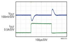
$\begin{array}{l} V_{IN}=5V, V_{OUT}=3.3V, f_{SW}=1MHz\\ C_{OUT}=2\times22\mu\text{F}\ CERAMIC\ CAP\\ C_{TH}=2200\text{pF}, R_{TH}=10k\\ \text{LOAD\ STEP\ 1A-2A} \end{array}$
