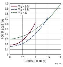
Figure 8. Power Loss at 5V Output and 1MHz Switching Frequency
