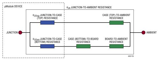
Figure 5. Graphical Representation of JESD51-12 Thermal Coefficients, Including JESD 51-12 Terms
