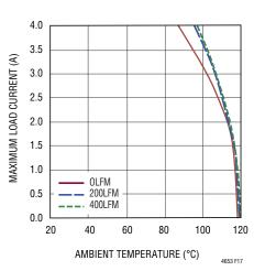
Figure 17. 12V to 1V<sub>OUT</sub> Derating Curve with BGA Heat Sink
