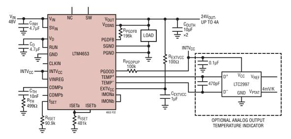
Figure 32. 4A, 24V Output DC/DC µModule Regulator
