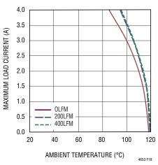
Figure 18. 24V to 1V<sub>OUT</sub> Derating Curve with BGA Heat Sink
