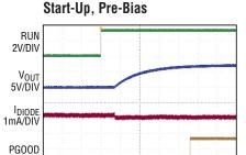
FIGURE 32 CIRCUIT,  $48V_{IN}$ ,  $C_{INH} = C_D = 4.7 \mu F$ ,  $C_{OUT} = 22 \mu F \times 2$ ,  $R_{fSET} = 124 k$ ,  $R_{ISET} = 240 k$ ,
