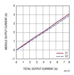
Figure 35. Current Sharing Performance of LTM4653s in Figure 34 Circuit
