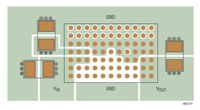
Figure 31. Recommend PCB Layout, Package Top View
