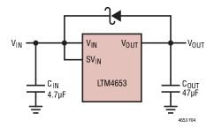
Figure 4. Schottky Diode from Volit to VIN
