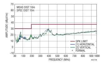
Figure 8. Radiated Emissions Scan of the LTM4653 Producing  $12V_{OUT}$  at 3A, from  $58V_{IN}$ , DC2327A Hardware,  $f_{SW}$  = 1.2MHz, Measured in a 10m Chamber, Peak Detect Method
