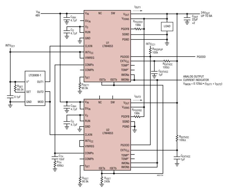
Figure 34. 24V Output at Up to 8A from 48V Input, 2-Phase Parallel with Analog Output Current Indicator
