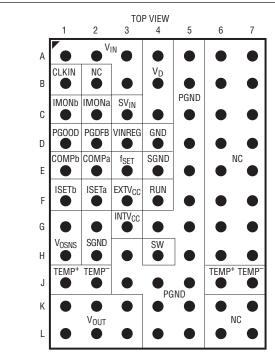
BGA PACKAGE 77-PIN (15mm × 9mm × 5.01mm)  $T_{J(MAX)} = 125$ °C;  $\theta_{JA} = 15.5$ °C/W;  $\theta_{\text{JCtop}} = 20.6^{\circ}\text{C/W}; \ \theta_{\text{JCbot}} = 5.1^{\circ}\text{C/W}; \ \text{WEIGHT} = 1.8 \ \text{GRAMS}$
