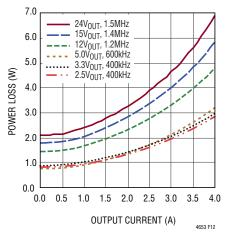
Figure 12. 48V<sub>IN</sub> Power Loss Curve
