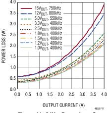
Figure 11. 24V<sub>IN</sub> Power Loss Curve
