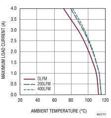
Figure 19. 12V to 5V<sub>OUT</sub> Derating Curve, No Heat Sink
