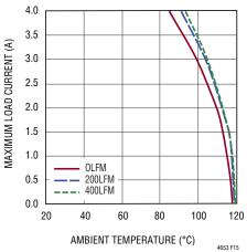
Figure 15. 24V to 1V<sub>OUT</sub> Derating Curve, No Heat Sink
