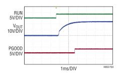
Figure 33. Start-Up Waveforms at  $48V_{IN}$ , Figure 32 Circuit
