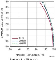
Figure 14. 12V to 1V<sub>OUT</sub> Derating Curve, No Heat Sink
