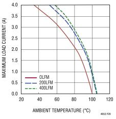
Figure 29. 48V to 15V<sub>OUT</sub> Derating Curve with BGA Heat Sink
