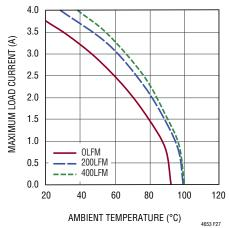
Figure 25. 24V to 15V<sub>OUT</sub> Derating Curve, No Heat Sink
