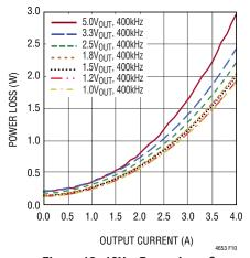
Figure 10. 12V<sub>IN</sub> Power Loss Curve
