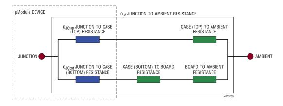
Figure 9. Graphical Representation of JESD51-12 Thermal Coefficients
