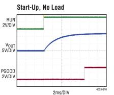
FIGURE 32 CIRCUIT,  $48V_{IN}$ ,  $C_{INH} = C_D = 4.7 \mu F$ ,  $C_{OUT} = 22 \mu F \times 2$ , R<sub>fSET</sub> = 124k, R<sub>ISET</sub> = 240k,  $R_{PGDFB} = 95.3k$  $C_{TH} = 10$ nF,  $R_{TH} = 562\Omega$ ,  $R_{\text{EXTVCC}} = 49.9\Omega$ ,  $C_{\text{EXTVCC}} = 1\mu\text{F}$ , NO LOAD
