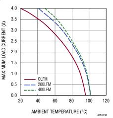
Figure 30. 48V to 24V<sub>OUT</sub> Derating Curve with BGA Heat Sink
