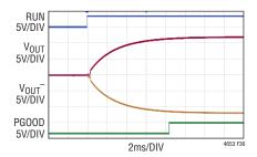
Figure 36. Concurrent ±12V Supply, Output Voltage Start-Up Waveforms, Figure 37 Circuit
