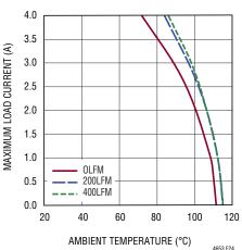
Figure 22. 12V to  $5V_{OUT}$  Derating Curve with BGA Heat Sink
