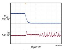
FIGURE 32 CIRCUIT,  $48V_{IN}$ ,  $C_{INH} = C_D = 4.7 \mu F$ ,  $C_{OUT} = 22 \mu F \times 2$ , R<sub>fSET</sub> = 124k, R<sub>ISET</sub> = 240k, R<sub>PGDFB</sub> = 95.3k,  $C_{TH} = 10$ nF,  $R_{TH} = 562\Omega$ ,  $R_{EXTVCC} = 49.9\Omega$ ,  $C_{EXTVCC} = 1\mu F$ , NO LOAD PRIOR TO APPLICATION OF OUTPUT SHORT-CIRCUIT
