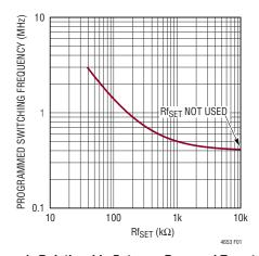
Figure 1. Relationship Between R<sub>fSET</sub> and Target f<sub>SW</sub>
