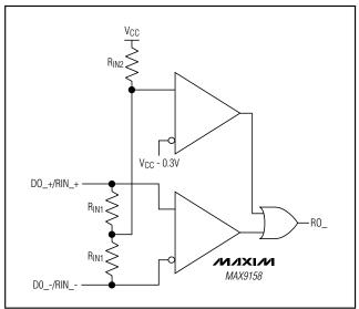
Figure 1. Internal Fail-Safe Circuit
