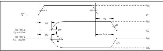
Figure 10. Receiver High-Impedance Waveforms
