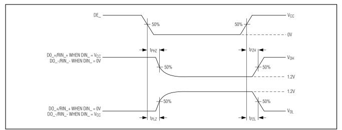
Figure 6. Driver High-Impedance Delay Waveform
