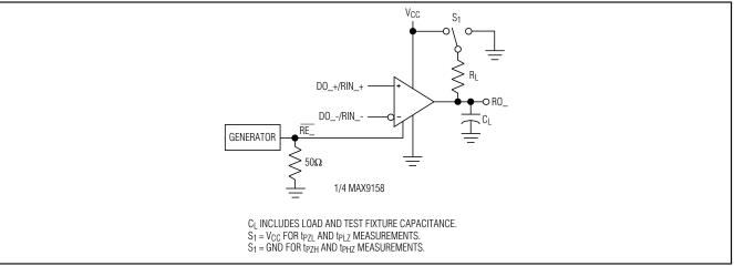
Figure 9. Receiver High-Impedance Delay Test Circuit
