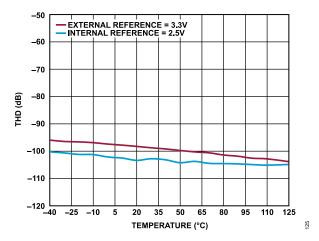
Figure 24. AD4683 THD vs. Temperature
