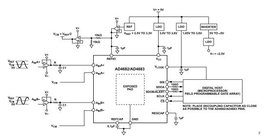
Figure 35. Typical Application Circuit
