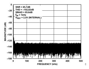
Figure 10. AD4682 FFT, V<sub>REF</sub> = 2.5 V Internal
