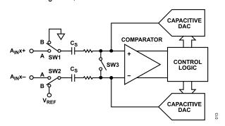
Figure 32. ADC Conversion Phase
