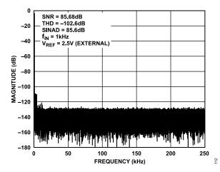
Figure 11. AD4683 FFT, V<sub>REF</sub> = 2.5 V External
