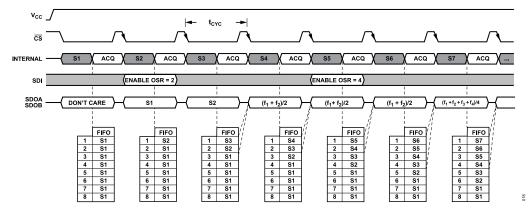
Figure 36. Rolling Average Oversampling Mode Configuration
