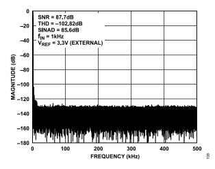
Figure 7. AD4682 Fast Fourier Transform (FFT), V<sub>REF</sub> = 3.3 V External
