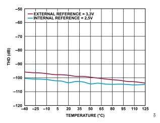
Figure 23. AD4682 THD vs. Temperature
