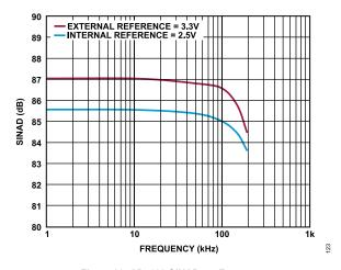
Figure 22. AD4683 SINAD vs. Frequency
