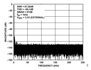
Figure 8. AD4683 FFT, V<sub>REF</sub> = 3.3 V External
