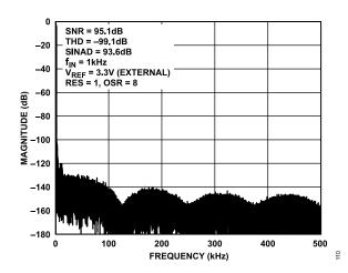
Figure 9. AD4682 FFT, Rolling Average Oversampling
