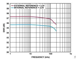
Figure 14. AD4682 SNR vs. Frequency
