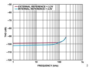
Figure 19. AD4683 THD vs. Frequency
