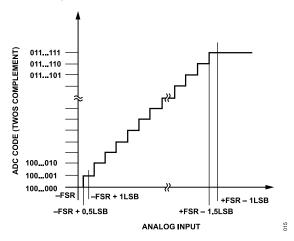
Figure 34. ADC Ideal Transfer Function (FSR = Full-Scale Range)
