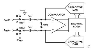
Figure 31. ADC Acquisition Phase
