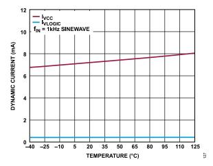
Figure 26. Dynamic Current vs. Temperature
