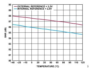
Figure 20. AD4682SNR vs. Temperature
