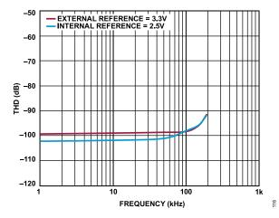
Figure 15. AD4682 THD vs. Frequency
