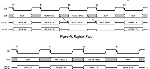
Figure 45. Register Write
