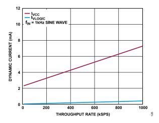
Figure 25. Dynamic Current vs. Throughput Rate
