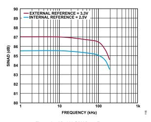
Figure 17. AD4682 SINAD vs. Frequency
