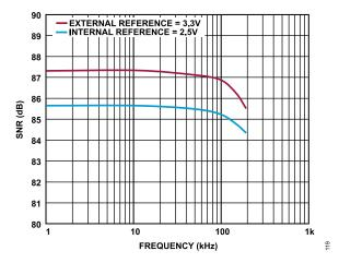
Figure 18. AD4683 SNR vs. Frequency
