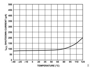
Figure 28. I<sub>VCC</sub> Shutdown Current vs. Temperature
