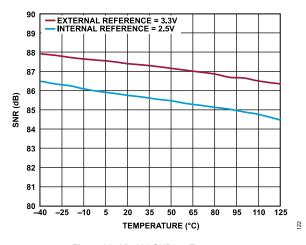
Figure 21. AD4683 SNR vs. Temperature
