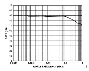
Figure 27. Power Supply Rejection Ratio (PSRR) vs. Ripple Frequency
