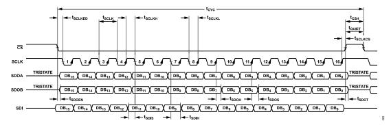
Figure 2. Serial Interface Timing Diagram
