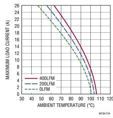
Figure 24. 12V to 1.8V Derating Curve, with Heat Sink
