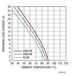
Figure 22. 24V to 1.8V Derating Curve, No Heat Sink
