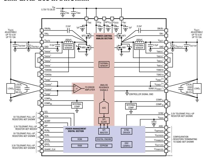
Figure 1. Simplified LTM4676A Block Diagram
