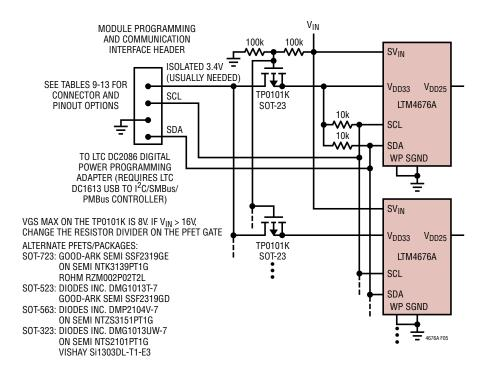
Figure 5. Circuit Suitable for Programming EEPROM/NVM of LTM4676A and Other ADI PSM Modules/ICs in Vast Systems, Even When  $V_{IN}$  Power is Absent,  $0^{\circ}C < T_{.I} \le 85^{\circ}C$
