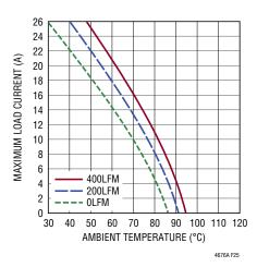
Figure 25. 24V to 1.8V Derating Curve, with Heat Sink
