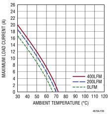
Figure 28. 24V to 3.3V Derating Curve. No Heat Sink
