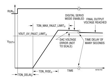
Figure 3. Timing Controlled Vout Rise
