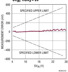
MFR\_READ\_IIN $_n$  (Input Current Readback) Error vs ( $I_{VIN}$  $_n$  +  $I_{SVIN}$ ), MFR\_PWM\_MODE $_n$ [0]=1 $_b$ ,  $I_{OUT}$  $_n$  Swept from 0A to 13A, One Channel at a Time, RUN $_{1-n}$  = 0V
