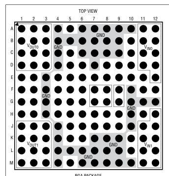
BGA PACKAGE 144-LEAD (16mm × 16mm × 5.01mm)
