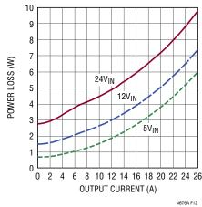
Figure 12. 1.8V<sub>OUT</sub> Power Loss Curve
