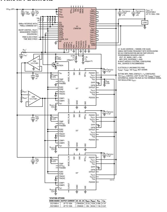
Figure 40. One LTM4676A Operating In Parallel with 3xLTM4620A or 3xLTM4630 (See Demo Boards DC2106B-A, DC2106B-B) Producing  $1V_{OUT}$  at up to  $100A \sim 130A$ . Power System Management Features Accessible Through LTM4676A. See Figure 41
