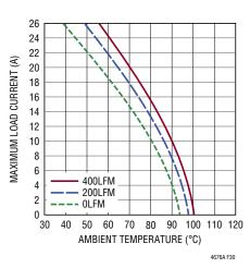
Figure 30. 12V to 3.3V Derating Curve, with Heat Sink
