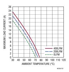
Figure 31. 24V to 3.3V Derating Curve, with Heat Sink
