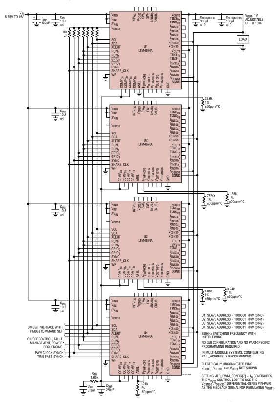
Figure 39. Four Paralleled LTM4676A Producing  $1V_{OUT}$  at Up to 100A. Integrated Power System Management Features Accessible Over 2-Wire  $I^2C/SMBus/PMBus$  Serial Interface. Evaluated on DC1989B-C
