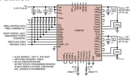
Figure 69. 13A, 1V and 13A, 1.8V Output DC/DC μModule Regulator with Serial Interface
