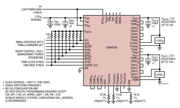
Figure 37. 13A, 1.2V and 2.5V Outputs Generated from 3.3V Power Input and Providing 12C/SMBus/PMBus Serial Interface
