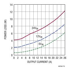
Figure 13. 3.3V<sub>OUT</sub> Power Loss Curve
