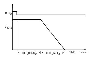
Figure 4. TOFF\_DELAY<sub>n</sub> and TOFF\_FALL<sub>n</sub>
