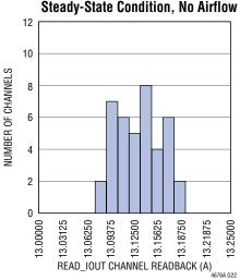
READ\_OUT of 20 LTM4676As (DC1811B-B) 12 $V_{IN}$ , 1 $V_{OUT}$ ,  $T_J = 125^{\circ}C$ ,  $I_{OUT,n} = 13A$ , System Having Reached Thermally Steady-State Condition. No Airflow
