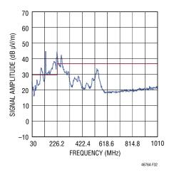
Figure 32. Radiated Emissions Scan of the LTM4676A Producing  $1V_{OUT}$  at 26A, from  $12V_{IN}$ . DC1811B-B Hardware with Outputs Paralleled. No Snubbers Applied.  $f_{SW} = 350$ kHz. Measured in a 10m Chamber. Peak Detect Method
