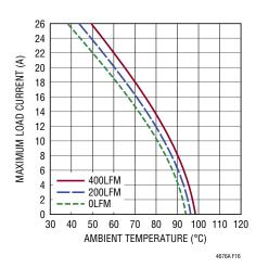
Figure 16. 24V to 1V Derating Curve, No Heat Sink
