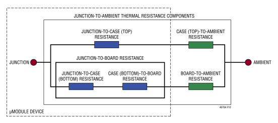
Figure 10. Graphical Representation of JESD51-12 Thermal Coefficients
