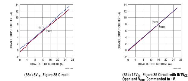
Figure 36. Current Sharing Performance of the LTM4676A's Channels
