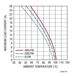
Figure 19. 24V to 1V Derating Curve, with Heat Sink
