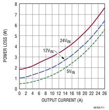
Figure 11. 1V<sub>OUT</sub> Power Loss Curve
