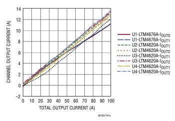
Figure 41a. LTM4676A Paralleled with 3x LTM4620A (Up to 100A Output)
