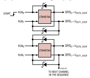
NOTE: RESISTOR OR RC PULL-UPS ON RUN, AND  $\overline{\text{GPIO}}_n$  PINS NOT SHOWN \*OPTIONAL SIGNAL SCHOTTKY DIODE. ONLY NEEDED WHEN ACCURATE PGOOD (POWER GOOD) INDICATION IS REQURED BY THE SYSTEM/USER IMMEDIATELY AT SVIN POWER UP
