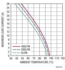
Figure 27. 12V to 3.3V Derating Curve, No Heat Sink
