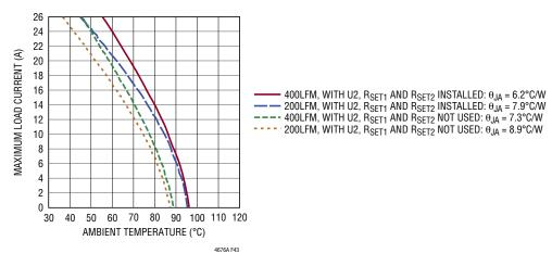
Figure 43. Output Derating Curve of Figure 42 Circuit Tested on DC1811B-B, 12V<sub>IN</sub>, No Heat Sink
