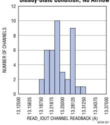
READ\_OUT of 20 LTM4676As (DC1811B-B) 12 $V_{IN}$ , 1 $V_{OUT}$ ,  $T_J = 25^{\circ}C$ ,  $I_{OUT}$ , = 13A, System Having Reached Thermally Steady-State Condition, No Airflow
