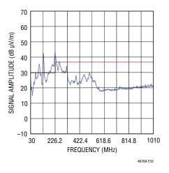
Figure 33. Radiated Emissions Scan of the LTM4676A Producing  $1V_{OUT}$  at 26A, from  $12V_{IN}$ . DC1811B-B Hardware with Outputs Paralleled.  $1\Omega$  (1/4W rated) Snubber Resistors Applied from SNUB<sub>n</sub> to GND.  $f_{SW}$  = 350kHz. Measured in a 10m Chamber. Peak Detect Method
