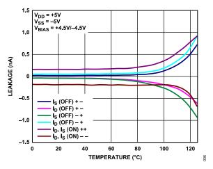
Figure 11. Leakage Currents vs. Temperature, ±5 V Dual Supply
