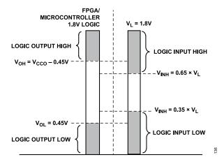
Figure 37. 1.8 V Logic Compatibility Between V<sub>OH</sub> and V<sub>OL</sub> and V<sub>INH</sub> and V<sub>INL</sub>
