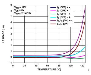
Figure 12. Leakage Currents vs. Temperature, 12 V Single Supply
