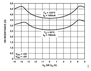
Figure 9. On Resistance vs.  $V_D$  or  $V_S$  for Different Current Levels, ±5 V Dual Supply
