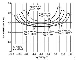
Figure 3. On Resistance vs. V<sub>D</sub> or V<sub>S</sub>, Dual Supply
