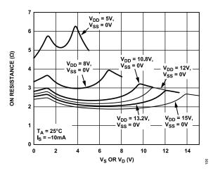
Figure 5. On Resistance vs. V<sub>D</sub> or V<sub>S</sub>, Single Supply
