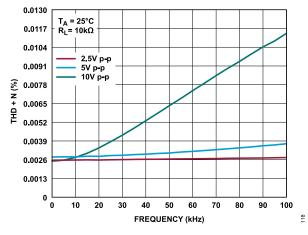
Figure 21. THD + N vs. Frequency, ±5 V Dual Supply
