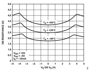
Figure 7. On Resistance vs.  $V_D$  or  $V_S$  for Different Temperatures, ±5 V Dual Supply
