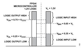
Figure 36. 1.2 V Logic Compatibility Between V<sub>OH</sub> and V<sub>OL</sub> and V<sub>INH</sub> and V<sub>INL</sub>
