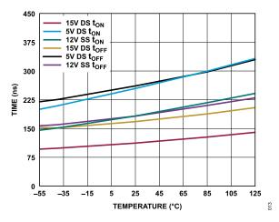
Figure 15. t<sub>ON</sub>/t<sub>OFF</sub> Time vs. Temperature for Single Supply (SS) and Dual Supply (DS)
