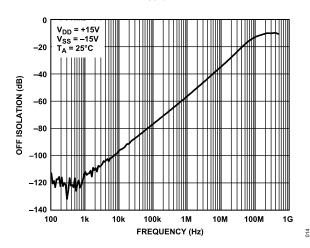
Figure 16. Off Isolation vs. Frequency, ±15 V Dual Supply
