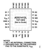
Figure 2. Pin Configuration
