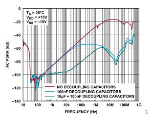
Figure 19. AC PSRR vs. Frequency, ±15 V Dual Supply
