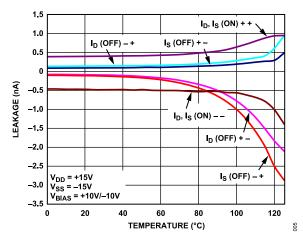
Figure 10. Leakage Currents vs. Temperature, ±15 V Dual Supply
