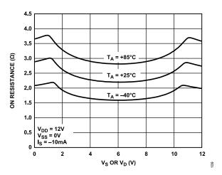
Figure 8. On Resistance vs. V<sub>D</sub> or V<sub>S</sub> for Different Temperatures, +12 V Single Supply
