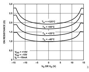
Figure 6. On Resistance vs. V<sub>D</sub> or V<sub>S</sub> for Different Temperatures,  $\pm$ 15 V Dual Supply
