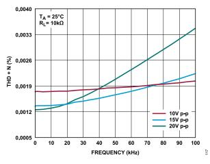
Figure 20. THD + N vs. Frequency, ±15 V Dual Supply
