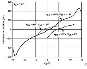
Figure 14. Charge Injection vs. V<sub>S</sub>
