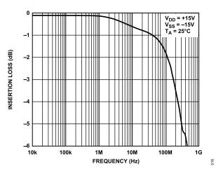
Figure 18. Insertion Loss vs. Frequency, ±15 V Dual Supply
