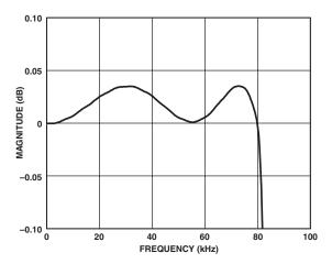
TPC 10. DAC Composite Filter Response,  $f_S = 192 \text{ kHz}$  (Pass-Band Section)
