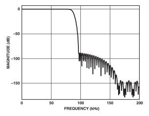
TPC 7. DAC Composite Filter Response,  $f_S = 192 \text{ kHz}$
