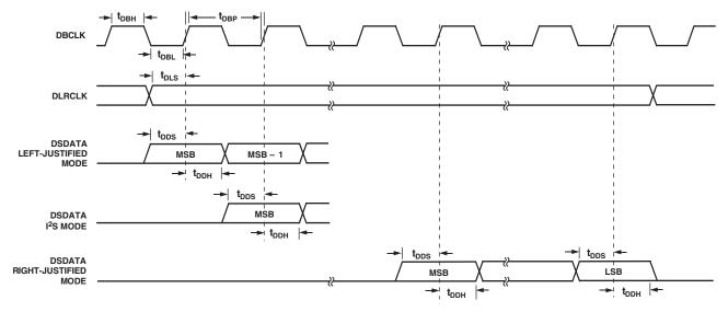
Figure 6. DAC Serial Mode Timing
