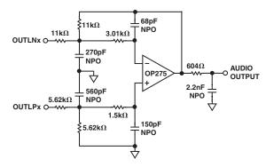
Figure 15. Typical DAC Output Filter Circuit
