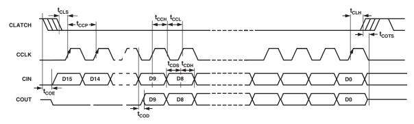
Figure 3. Format of SPI Timing
