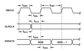
Figure 10. DAC Packed Mode Timing
