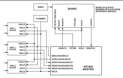
Figure 12. Aux Mode Connection to SHARC (Master Mode)
