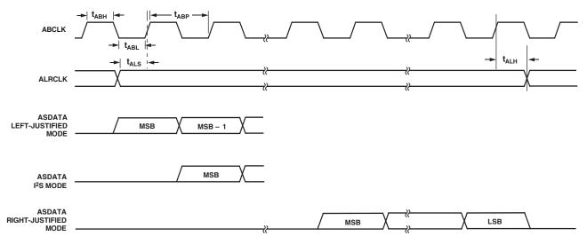
Figure 5. ADC Serial Mode Timing
