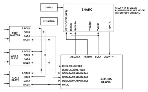
Figure 13. Aux Mode Connection to SHARC (Slave Mode)
