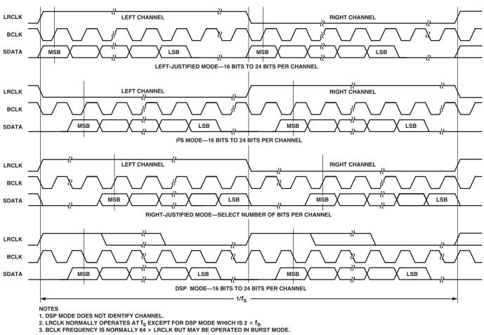
Figure 4. Stereo Serial Modes
