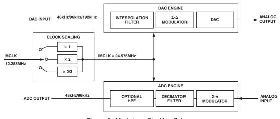
Figure 2. Modulator Clocking Scheme
