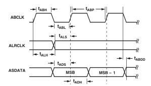
Figure 9. ADC Packed Mode Timing
