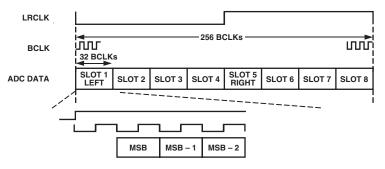
Figure 7. ADC Packed Mode 256
