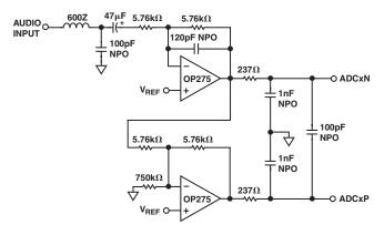
Figure 14. Typical ADC Input Filter Circuit
