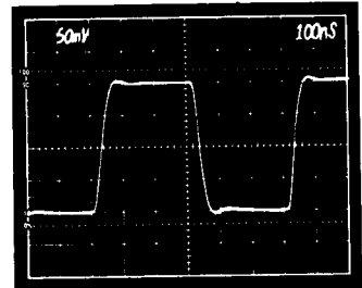
Figure 22c. Unity Gain Follower Small Signal Pulse Response, C_{COMP} = 5pF
