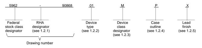
1.2.1 <u>RHA designator</u>. Device classes Q and V RHA marked devices meet the MIL-PRF-38535 specified RHA levels and are marked with the appropriate RHA designator. Device class M RHA marked devices meet the MIL-PRF-38535, appendix A specified RHA levels and are marked with the appropriate RHA designator. A dash (-) indicates a non-RHA device.
