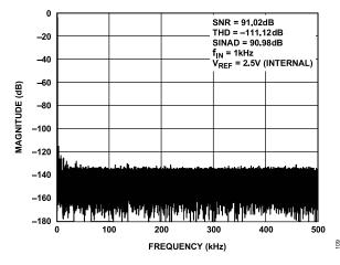
Figure 7. AD4680 Fast Fourier Transform (FFT), V<sub>REF</sub> = 2.5 V Internal
