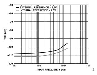
Figure 22. AD4681 THD vs. Input Frequency
