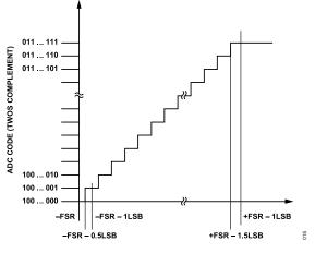
Figure 31. ADC Ideal Transfer Function (FSR = Full-Scale Range)
