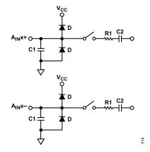
Figure 30. Equivalent Analog Input Circuit, Conversion Phase—Switches Open, Track Phase—Switches Closed
