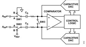
Figure 29. ADC Conversion Phase
