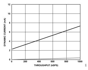
Figure 21. Dynamic Current vs. Throughput
