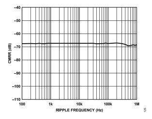
Figure 27. CMRR vs. Ripple Frequency
