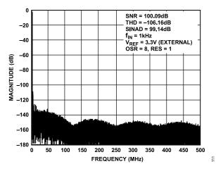
Figure 9. AD4680 FFT with Oversampling, V<sub>REF</sub> = 3.3 V External
