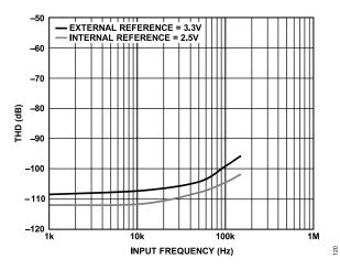
Figure 18. AD4680 THD vs. Input Frequency
