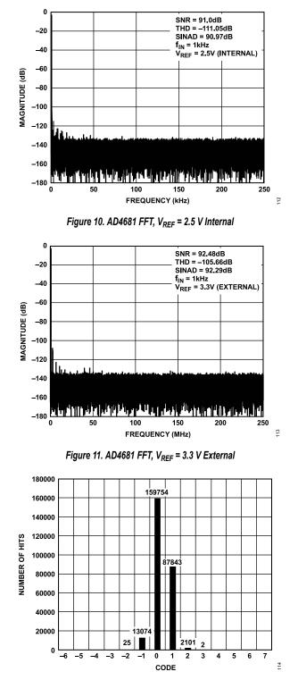
Figure 12. DC Histogram Codes at Code Center
