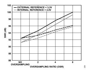
Figure 24. AD4680 SNR vs. Oversampling Ratio, Oversampling Mode
