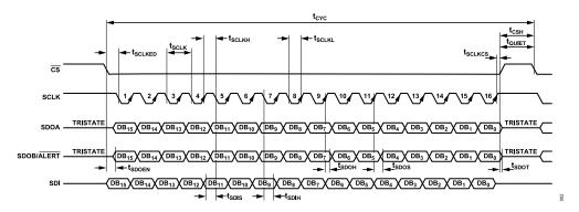
Figure 2. Serial Interface Timing Diagram
