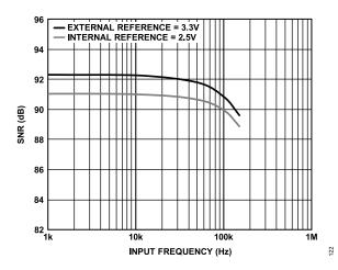
Figure 20. AD4681 SNR vs. Input Frequency
