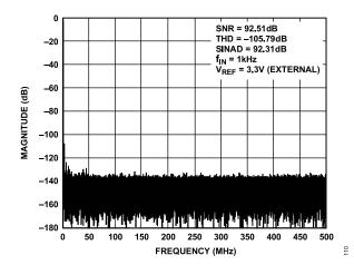
Figure 8. AD4680 FFT, V<sub>REF</sub> = 3.3 V External
