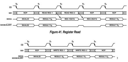
Figure 42. Register Write
