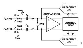
Figure 28. ADC Acquisition Phase
