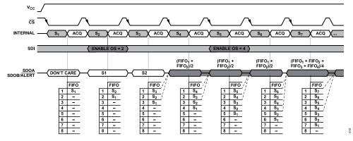
Figure 33. Rolling Average Oversampling Operation
