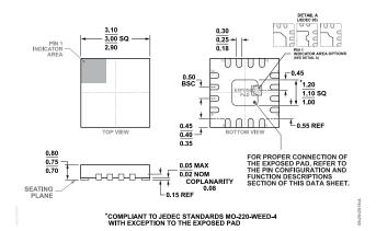
Figure 44. 16-Lead Lead Frame Chip Scale Package [LFCSP] 3 mm × 3 mm Body and 0.75 mm Package Height (CP-16-45) Dimensions shown in millimeters
