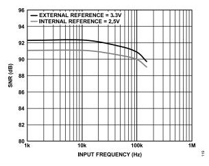
Figure 17. AD4680 SNR vs. Input Frequency
