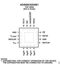
Figure 6. Pin Configuration
