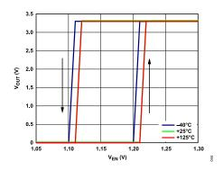
Figure 46. Typical VOUT Response to EN Pin Operation
