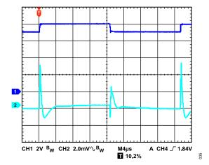
Figure 37. Line Transient Response,  $I_{LOAD}$  = 200 mA,  $V_{OUT}$  = 5 V, CH1  $V_{IN}$ , CH2  $V_{OUT}$
