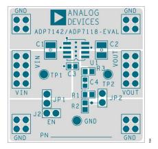
Figure 65. Example SOIC PCB Layout
