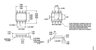
Figure 68. 8-Lead Standard Small Outline Package, with Exposed Pad [SOIC\_N\_EP]
