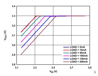
Figure 23. Output Voltage ( $V_{OUT}$ ) vs. Input Voltage ( $V_{IN}$ ) in Dropout,  $V_{OUT}$  = 3.3 V
