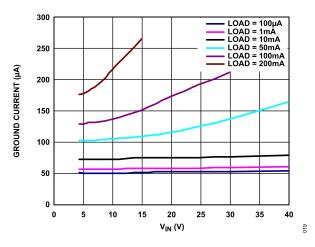
Figure 21. Ground Current ( $I_{GND}$ ) vs. Input Voltage ( $V_{IN}$ ),  $V_{OUT}$  = 3.3 V
