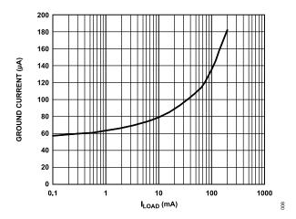
Figure 10. Ground Current (I<sub>GND</sub>) vs. Load Current (I<sub>LOAD</sub>)
