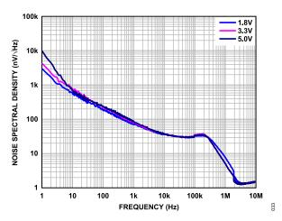
Figure 35. Output Noise Spectral Density vs. Frequency, for Different Output Voltages ( $V_{OUT}$ )
