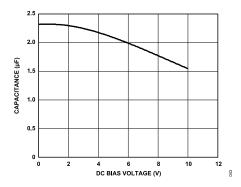
Figure 45. Capacitance vs. Voltage Characteristic
