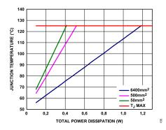
Figure 56. SOIC,  $T_A = 50$ °C
