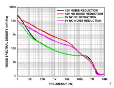
Figure 51. 6 V and 12 V Output Voltage with and Without Noise Reduction Network
