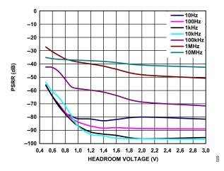
Figure 31. Power Supply Rejection Ratio (PSRR) vs. Headroom Voltage,  $V_{OUT}$  = 5 V, for Different Frequencies
