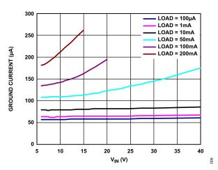
Figure 11. Ground Current ( $I_{GND}$ ) vs. Input Voltage ( $V_{IN}$ )
