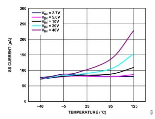
Figure 25. Soft Start (SS) Current vs. Temperature  $(T_J)$ , Multiple Input Voltages  $(V_{IN})$ ,  $V_{OUT} = 5 V$
