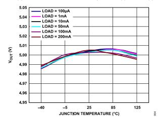
Figure 6. Output Voltage (V<sub>OUT</sub>) vs. Junction Temperature (T<sub>J</sub>)
