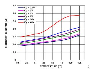
Figure 12. Shutdown Current ( $I_{\rm GND-SD}$ ) vs. Temperature at Various Input Voltages ( $V_{\rm IN}$ )
