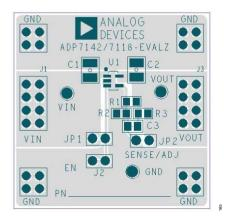
Figure 66. Example TSOT PCB Layout
