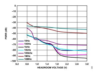
Figure 27. Power Supply Rejection Ratio (PSRR) vs. Headroom Voltage,  $V_{OUT}$  = 1.8 V, for Different Frequencies
