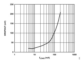
Figure 13. Dropout Voltage ( $V_{DROPOUT}$ ) vs. Load Current ( $I_{LOAD}$ ),  $V_{OUT} = 5 \text{ V}$
