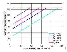
Figure 63. TSOT Junction Temperature Rise, Different Board Temperatures
