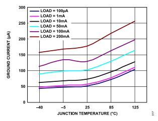
Figure 19. Ground Current ( $I_{GND}$ ) vs. Junction Temperature ( $T_J$ ),  $V_{OUT} = 3.3 \text{ V}$
