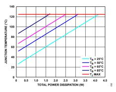
Figure 55. SOIC,  $T_A = 25$ °C
