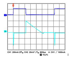
Figure 36. Load Transient Response,  $I_{LOAD}$  = 1 mA to 200 mA,  $V_{OUT}$  = 5 V,  $V_{IN}$  = 7 V, CH1 Load Current ( $I_{LOAD}$ ), CH2  $V_{OUT}$
