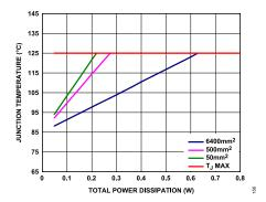
Figure 57. SOIC,  $T_A = 85^{\circ}\text{C}$
