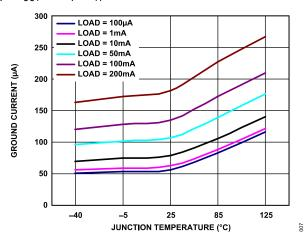
Figure 9. Ground Current (I<sub>GND</sub>) vs. Junction Temperature (T<sub>J</sub>)
