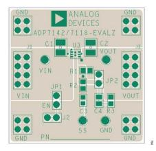
Figure 64. Example LFCSP PCB Layout
