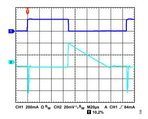
Figure 40. Load Transient Response,  $I_{LOAD}$  = 1 mA to 200 mA,  $V_{OUT}$  = 1.8 V,  $V_{IN}$  = 3 V, CH1 Load Current ( $I_{LOAD}$ ), CH2  $V_{OUT}$
