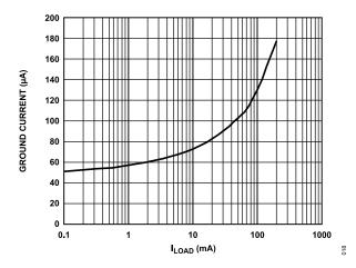
Figure 20. Ground Current ( $I_{GND}$ ) vs. Load Current ( $I_{LOAD}$ ),  $V_{OUT}$  = 3.3 V
