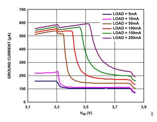
Figure 24. Ground Current ( $I_{GND}$ ) vs. Input Voltage ( $V_{IN}$ ) in Dropout,  $V_{OUT}$  = 3.3 V
