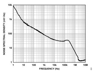
Figure 33. Output Noise Spectral Density vs. Frequency,  $I_{LOAD} = 10 \text{ mA}$
