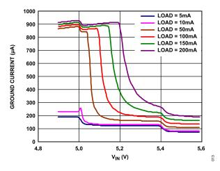
Figure 15. Ground Current ( $I_{GND}$ ) vs. Input Voltage ( $V_{IN}$ ) in Dropout,  $V_{OUT}$  = 5 V
