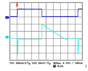
Figure 38. Load Transient Response,  $I_{LOAD}$  = 1 mA to 200 mA,  $V_{OUT}$  = 3.3 V,  $V_{IN}$  = 5 V, CH1 Load Current ( $I_{LOAD}$ ), CH2  $V_{OUT}$
