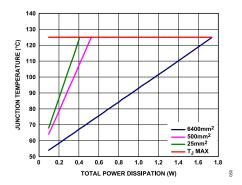
Figure 53. LFCSP,  $T_A = 50$ °C
