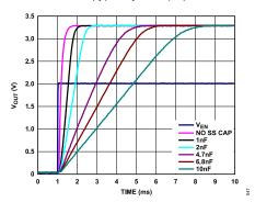
Figure 49. Typical Soft Start Behavior, Different C<sub>SS</sub>
