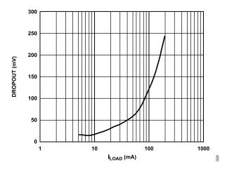
Figure 22. Dropout Voltage ( $V_{DROPOUT}$ ) vs. Load Current ( $I_{LOAD}$ ),  $V_{OUT}$  = 3.3 V
