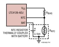
Figure 14. NTC Thermistor Connection
