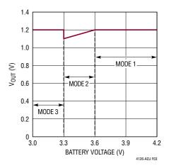
Figure 3.  $V_{OUT}$  vs Battery Voltage at  $I_{OUT} = 0$
