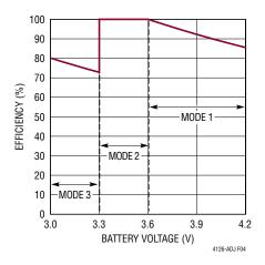
Figure 4. Theoretical Maximum Converter Efficiency vs Battery Voltage
