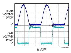
Figure 10. Voltage on the Drain and Gate of NMOS M1 when  $f_{TX\ TANK}$  = 1.29  $\bullet$   $f_{DRIVE}$
