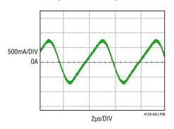
Figure 8. Current Through Transmit Coil
