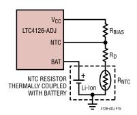
Figure 15. NTC Thermistor Connection with Desensitizing Resistor  $R_{\text{D}}$
