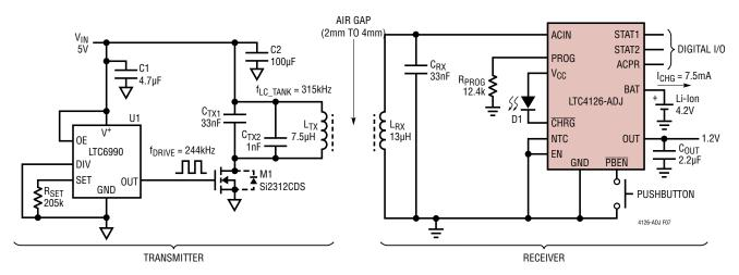
Figure 7. DC/AC Converter, Transmit/Receive Coil, Tuned Resonant LTC4126-ADJ Receiver (See Table 4 and Table 5 for Recommended Components)
