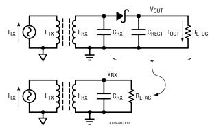
Figure 12. Modeling Parallel Resonant Configuration and Half Wave Rectifier on the Receiver
