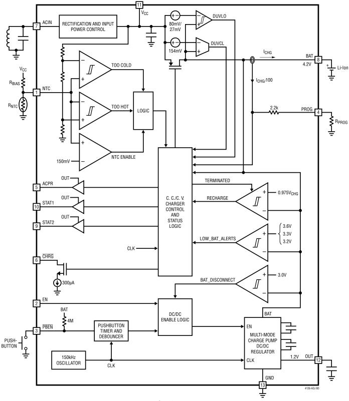
Figure 1. LTC4126-ADJ Block Diagram
