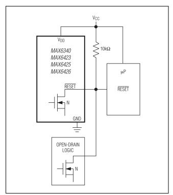
Figure 2. Wired-OR Reset Circuit
