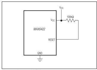
Figure 4. Ensuring RESET Valid to  $V_{CC} = 0$
