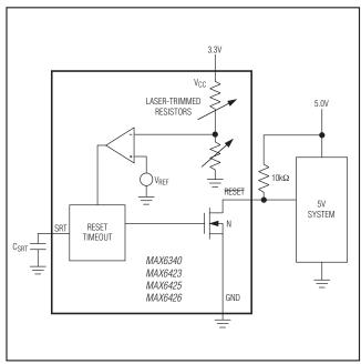
Figure 1. MAX6340/MAX6423/MAX6425/MAX6426 Open-Drain RESET Output Allows Use with Multiple Supplies
