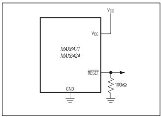
Figure 3. Ensuring  $\overline{RESET}$  Valid to  $V_{CC} = 0$
