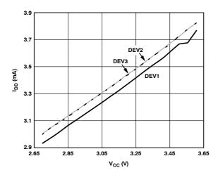
Figure 6. Supply Current vs. Voltage
