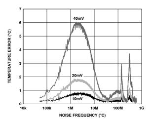
Figure 12. Temperature Error vs. Differential-Mode Noise Frequency
