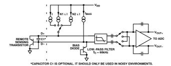
Figure 14. Signal Conditioning for Remote Diode Temperature Sensors
