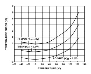
Figure 7. Remote Temperature Error
