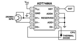
Figure 18. ADT7486A Typical Application Schematic
