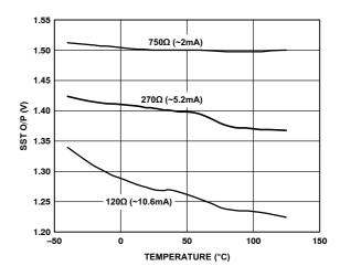
Figure 5. SST O/P Level vs. Temperature
