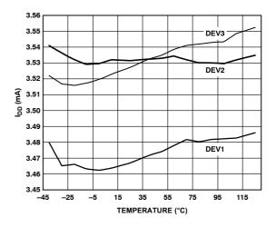
Figure 3. Supply Current vs. Temperature
