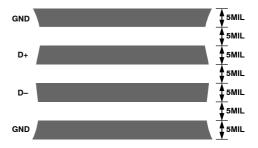
Figure 16. Arrangements of Signal Tracks
