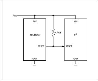
Figure 5. Interfacing to μPs with Bidirectional Reset I/O
