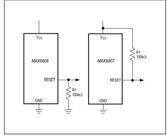
Figure 4.  $\overline{RESET}$  / RESET Valid to  $V_{CC}$  = Ground Circuit
