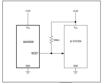
Figure 1. The MAX6808 Open-Drain RESET Output Allows Use with Multiple Supplies
