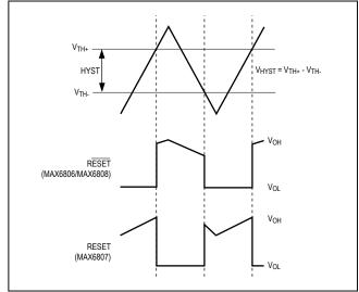
Figure 2. Input and Output Waveforms with V<sub>CC</sub> Varied
