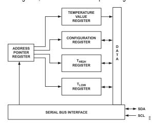
Figure 8. AD7414 Register Structure
