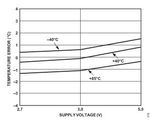
Figure 16. Typical Temperature Error vs. Supply for Large Sample of Parts
