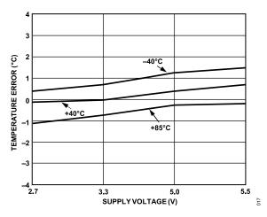
Figure 17. Typical Temperature Error vs. Supply for One Part
