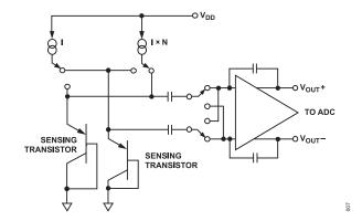
Figure 7. Temperature Measurement Technique
