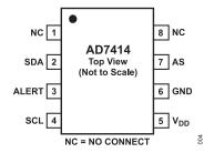
Figure 4. AD7414 Pin Configuration (MSOP)
