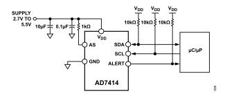
Figure 6. Typical Connection Diagram
