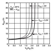
TPC 1. On Resistance vs. Input Voltage
