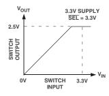
Figure 6. 3.3 V to 2.5 V Voltage Translation,  $\overline{SEL} = V_{CC}$
