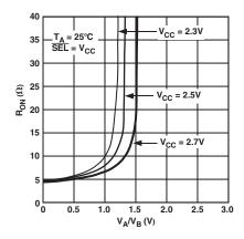
TPC 2. On Resistance vs. Input Voltage
