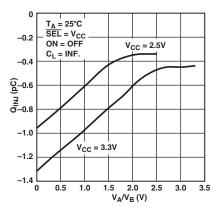
TPC 12. Charge Injection vs. Source Voltage
