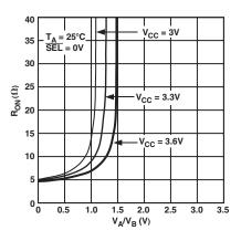
TPC 3. On Resistance vs. Input Voltage
