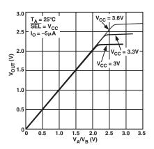
TPC 6. Pass Voltage vs.  $V_{CC}$
